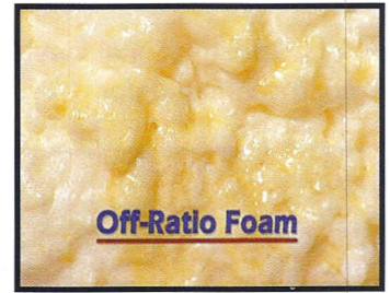
More "A" chemical is being dispensed
